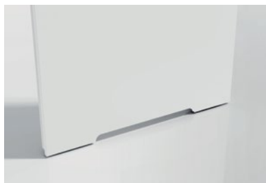
VENTILATION UNDERCUT IN PANEL DOORS 1 undercut 15 mm – for rooms with recuperation undercut 26 mm – WC for doors 80'-100' undercut 38 mm – WC for doors 60'-70'
