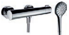
HF905451100600 Thermostatic shower mixer, fittings distance 134–166 mm, with fittings, with synthetic flexible hose 1500 mm, with handspray MyTwin100, chrome
