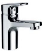
HF500942100000 Basin mixer, projection 110 mm, fixed spout, Eco+ function, without pop-up waste, chrome
