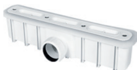
LAUFEN PRO S H290182 Linear siphon for PRO S shower trays with water trap height of 30 mm
