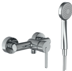
LUA H331081...1311 Shower mixer, fittings distance 134–166 mm, with fittings, with synthetic flexible hose 1600 mm, with handspray Stella 80 1F
