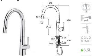
Electronic single-lever kitchen mixer with retractable swivel spout, 2-function rinse spray function and flexible supply hoses. Cold start. Mains operated at 230V. Power source included.
